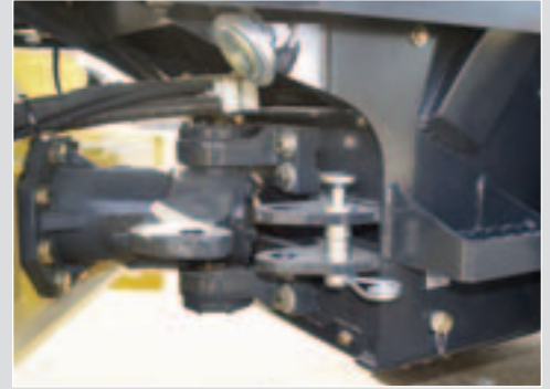
Bolt-on centerjoint is maintenance-free
